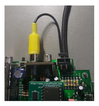
3. Both the SCART connector and the HDMI adapter require power connect as shown below.
